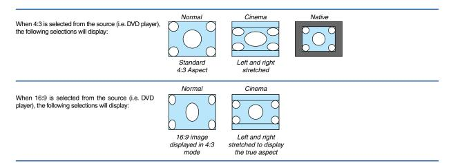
Native (RGB only): Turns off the scaling feature. The projector displays the current image in its true resolution.
